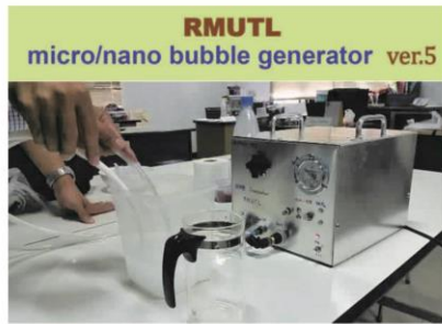
Fig.2. KVM01, flow rate of 1 L/min based on pressurized dissolved gas method developed by RMUTL.
