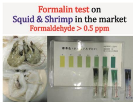
Fig. 1. Formaldehyde pack test results for shrimps and squids from fish market in the northern Thailand. From left, shrimps, squids, 2 ppm HCHO, and original HCHO.
